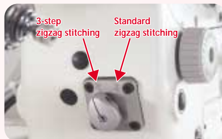
Standard/3-step zigzag stitching pattern changeover lever
